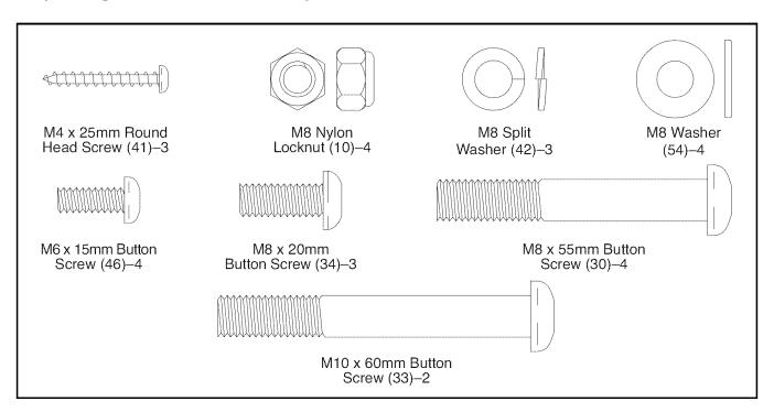
1. Slide the Rear Stabilizer (6) into the Frame (1). Attach the Rear Stabilizer with four M8 x 55mm Button Screws (30).
